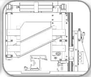
**With this special version** of the cutting blade head, the cutting blade may be applied in two positions. In this way, corresponding application of the blade may be adjusted to match the angle to the characteristics of the respective profile geometry. An additional advantage of this version of the profile guillotine is that only one guide column is used to fasten the cutting blade head.
